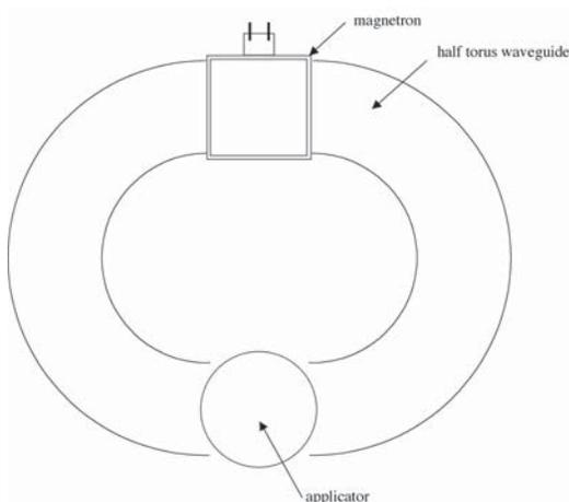
Fig. 1. RIMM circuit including the magnetron, the applicator connected with two half tours wave guides.
