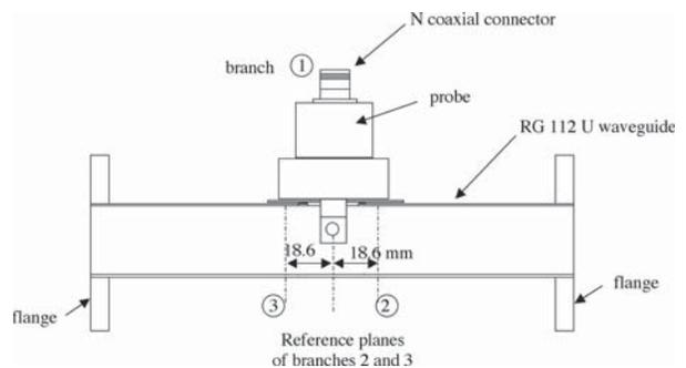
Fig. 2. Bi-directional magnetron waveguide launcher with a probe placed instead of the magnetron.
