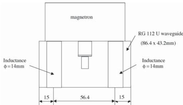
Fig. 3. Matching inductance of a bi-directional waveguide launcher, with inductance stubs.
