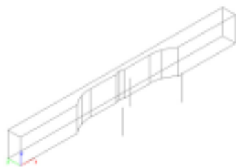
Fig. 3. Shape of the xylophone-beam of length 31 cm with two cutoffs, the large first cutoff and the small second cutoff in the middle. The length from top to the beginning of the cutoff is 8,2 cm, the curvature of the cutoff 3,0 cm, the way to the second cutoff in the middle is 3,7 cm, the second cutoff is 1,2 cm. The curvature is \sin(x)^p .
