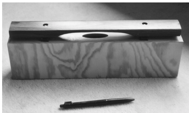
The used xylophone beam made of Palisol, which is a substitute for the rare wood Palisander.
