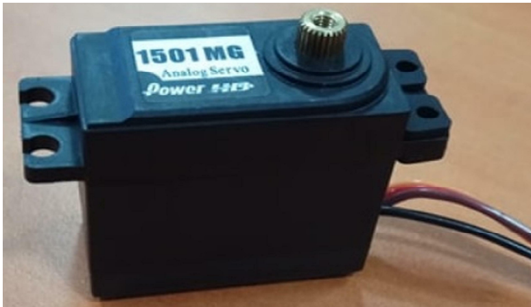
Fig. 8. Servomotor RC Power HD High-Torque Servo 1501MG .
